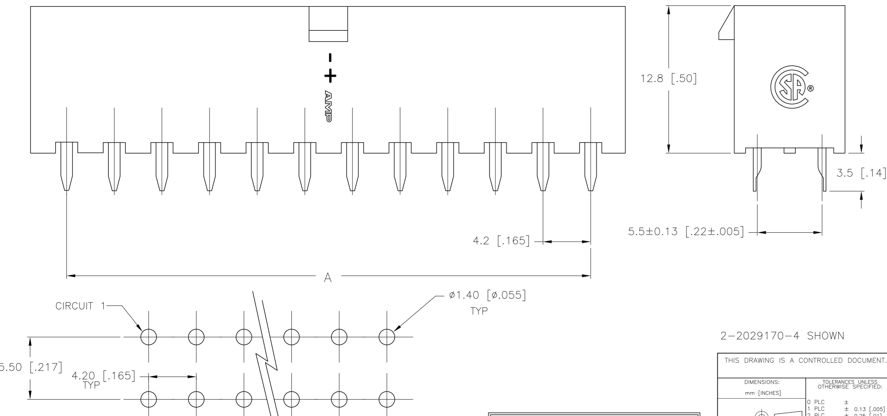
PCB LAYOUT: COMPONENT SIDE
