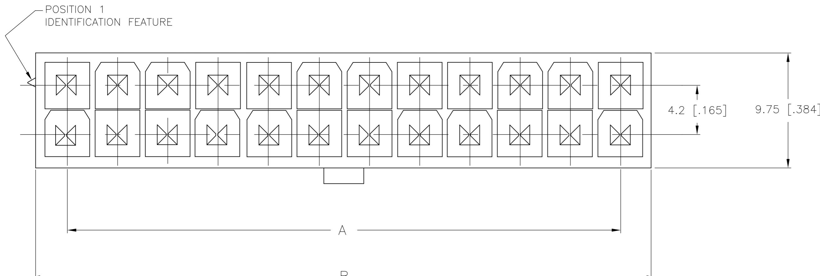
1 MATERIAL: HOUSING: NYLON, UL94V-2
