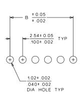
PCB LAYOUT: COMPONENT SIDE RECOMMENDED PCB THICKNESS:  $\frac{1.57 \pm 0.18}{.062 \pm .007}$
