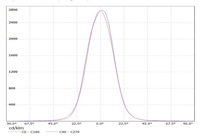
Luminaire: LEDIL OY CP12672\_TINA2-M (XB-D) Efficiency=82% Lamps: 1 x Cree XB-D white (97Im @ 250mA)
