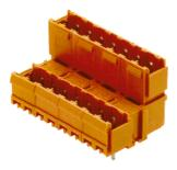
Dimensionally stable, straight, codable 2-tier male connector from the Unimate range of plugs with integral aid to prevent wrong connections. Available with open or closed sides. Fixing blocks can be attached to the closed version. The solder pin length of 3.2 mm has been optimised for wave soldering. Supplied in cardboard box.
