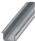
DIN rail, unperforated, Standard profile, width: 35 mm, height: 15 mm, similar to EN 60715: 2001, material: Steel, galvanized, length: 2000 mm, color: silver
