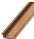
DIN rail, unperforated, Standard profile, width: 35 mm, height: 7.5 mm, In acc. with EN 60715: 2001, material: Copper, uncoated, length: 2000 mm, color: copper-colored
