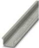
DIN rail, unperforated, Standard profile 2.3 mm, width: 35 mm, height: 15 mm, In acc. with EN 60715: 2001, material: Steel, galvanized, passivated with a thick layer, length: 2000 mm, color: silver
