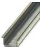
DIN rail, unperforated, Standard profile, width: 35 mm, height: 15 mm, similar to EN 60715: 2001, material: Steel, galvanized, passivated with a thick layer, length: 2000 mm, color: silver
