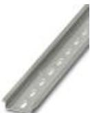
DIN rail perforated, Standard profile, width: 35 mm, height: 7.5 mm, In acc. with EN 60715: 2001, material: Steel, galvanized, passivated with a thick layer, length: 2000 mm, color: silver
