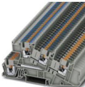
Installation level terminal block, Push-in connection, cross section: 0.14 mm<sup>2</sup> - 4 mm<sup>2</sup>, AWG: 26 - 12, width: 5.2 mm, color: gray, mounting type: NS 35/7,5, NS 35/15
