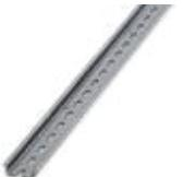
DIN rail perforated, Standard profile, width: 35 mm, height: 7.5 mm, In acc. with EN 60715: 2001, material: Steel, Galvanized, white passivated, length: 2000 mm, color: white
