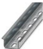
DIN rail perforated, Standard profile, width: 35 mm, height: 15 mm, similar to EN 60715: 2001, material: Steel, galvanized, length: 2000 mm, color: silver
