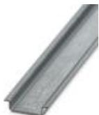
DIN rail, unperforated, Standard profile, width: 35 mm, height: 7.5 mm, In acc. with EN 60715: 2001, material: Steel, galvanized, length: 2000 mm, color: silver
