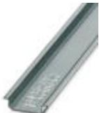
DIN rail, unperforated, Standard profile, width: 35 mm, height: 7.5 mm, In acc. with EN 60715: 2001, material: Steel, Galvanized, white passivated, length: 2000 mm, color: white
