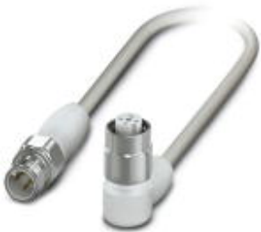
Sensor/Actuator cable, 4-position, PP-EPDM halogen-free, Gray RAL 7035, Plug straight M12, A-coded, on Socket angled M12, A-coded, with 3 LEDs, Cable length: 1.5 m, Hygienic design, With high-grade steel knurl
