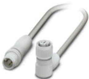
Sensor/Actuator cable, 4-position, PP-EPDM halogen-free, Gray RAL 7035, Plug straight M12, A-coded, on Socket angled M12, A-coded, with 3 LEDs, Cable length: 1.5 m, Hygienic design, with plastic knurl
