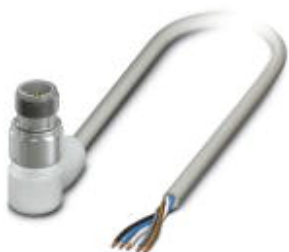
Sensor/Actuator cable, 5-position, PP-EPDM halogen-free, Gray RAL 7035, Plug angled M12, A-coded, on free cable end, Cable length: 3 m, Hygienic design, With high-grade steel knurl
