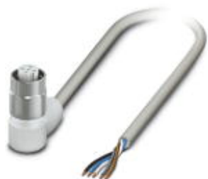
Sensor/Actuator cable, 5-position, PP-EPDM halogen-free, Gray RAL 7035, free cable end, on Socket angled M12, A-coded, with 3 LEDs, Cable length: 10 m, Hygienic design, With high-grade steel knurl
