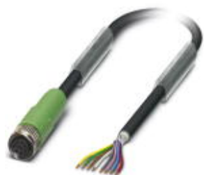
Sensor/Actuator cable, 8-position, PUR halogen-free, Black RAL 9005, shielded, free cable end, on Socket straight M8, Cable length: 10 m
