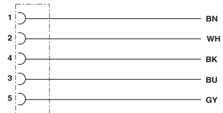
Contact assignment of the M12 socket
