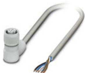
Sensor/Actuator cable, 5-position, PP-EPDM halogen-free, Gray RAL 7035, free cable end, on Socket angled M12, A-coded, Cable length: 3 m, Hygienic design, with plastic knurl
