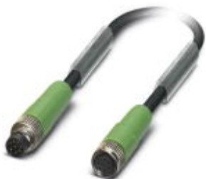
Sensor/Actuator cable, 8-position, PUR halogen-free, Black RAL 9005, Plug straight M8, on Socket straight M8, Cable length: 0.6 m
