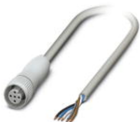
Sensor/Actuator cable, 5-position, PP-EPDM halogen-free, Gray RAL 7035, free cable end, on Socket straight M12, A-coded, Cable length: 3 m, Hygienic design, with plastic knurl
