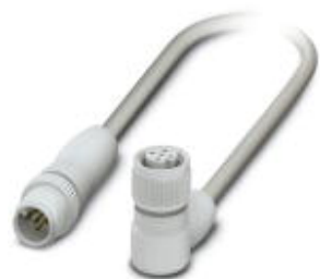
Sensor/Actuator cable, 5-position, PP-EPDM halogen-free, Gray RAL 7035, Plug straight M12, A-coded, on Socket angled M12, A-coded, with 3 LEDs, Cable length: 0.3 m, Hygienic design, with plastic knurl
