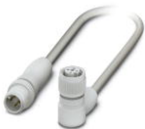
Sensor/Actuator cable, 4-position, PP-EPDM halogen-free, Gray RAL 7035, Plug straight M12, A-coded, on Socket angled M12, A-coded, Cable length: 0.3 m, Hygienic design, with plastic knurl
