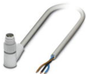
Sensor/Actuator cable, 3-position, PP-EPDM halogen-free, Gray RAL 7035, Plug angled M8, on free cable end, Cable length: 1.5 m, Hygienic design, with plastic knurl
