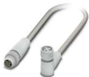
Sensor/Actuator cable, 3-position, PP-EPDM halogen-free, Gray RAL 7035, Plug straight M8, on Socket angled M8, with 2 LEDs, Cable length: 1.5 m, Hygienic design, with plastic knurl
