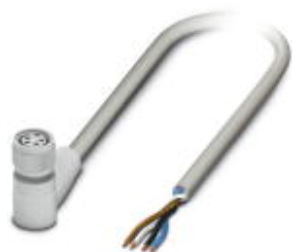
Sensor/Actuator cable, 4-position, PP-EPDM halogen-free, Gray RAL 7035, free cable end, on Socket angled M8, Cable length: 5 m, Hygienic design, with plastic knurl
