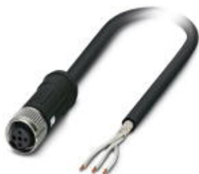
Sensor/Actuator cable, 3-position, RADOX® GKW S halogen-free, black, shielded, free cable end, on Socket straight M12 SPEEDCON, A-coded, Cable length: 2 m, For railway applications
