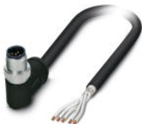
Sensor/Actuator cable, 5-position, RADOX® GKW S halogen-free, black, shielded, Plug angled M12 SPEEDCON, A-coded, on free cable end, Cable length: 10 m, For railway applications
