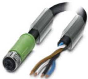
Power cable, 4-position, PUR halogen-free, black-gray RAL 7021, free cable end, on Socket straight M12 SPEEDCON, T-coded, Cable length: 10 m, for direct current up to 12 A/60 V
