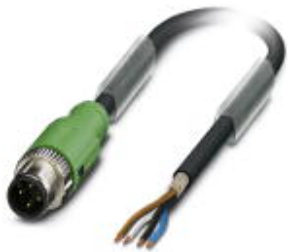
Sensor/Actuator cable, 4-position, PUR halogen-free, black-gray RAL 7021, shielded, Plug straight M12 SPEEDCON, A-coded, on free cable end, Cable length: 1.5 m
