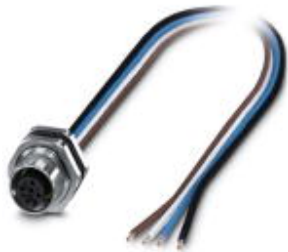
Bus system flat-type plug, 4-position, SocketLink:M12, D-coded, Rear mounting, M16 x 1.5, Individual wires, Cable length: 0.5 m
