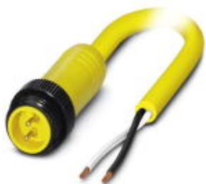
Power cable, 2-position, PVC, yellow, Plug straight 7/8"-16UNF, A - standard, on free cable end, cable length: 5 m
