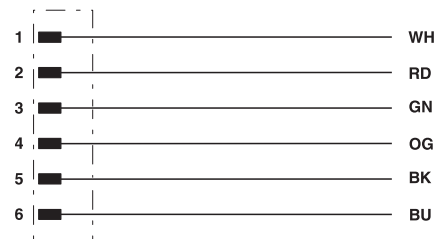
Contact assignment of 7/8" plug
