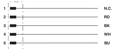
Contact assignment of 7/8" plug
