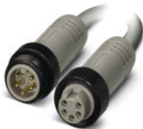
Bus system cable, DeviceNet™, 5-position, PVC, gray, Plug straight 7/8"-16UNF, A - standard, on Socket straight 7/8"-16UNF, cable length: 20 m
