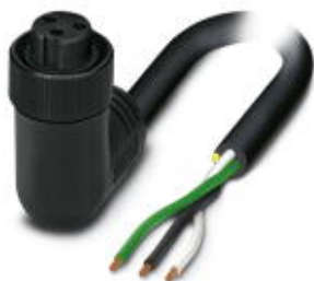
Power cable, 3-position, PVC, black, free cable end, A - standard, on Socket angled 7/8"-16UNF, Cable length: 2 m
