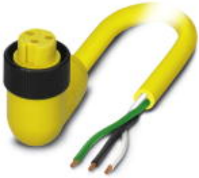
Power cable, 3-position, PVC, yellow, free cable end, A - standard, on Socket angled 7/8"-16UNF, Cable length: 10 m
