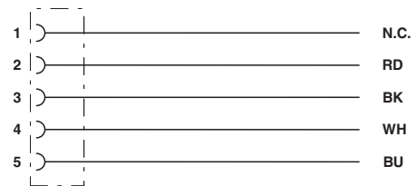
Contact assignment of 7/8" socket
