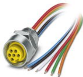
Sensor/actuator flush-type plug, 6-pos., 7/8", front mounting with 7/8" fastening thread, with 1.0 m PE litz wire
