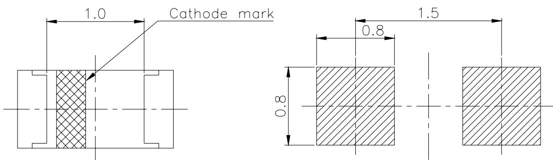
**Note:** The tolerances unless mentioned is ±0.1mm ,Unit = mm
