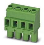
Plug component, Nominal current: 12 A, Rated voltage (III/2): 630 V, Number of positions: 4, Pitch: 7.62 mm, Connection method: Screw connection with tension sleeve, Color: green, Contact surface: Tin
