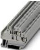
Feed-through terminal block, Connection type: Spring-cage connection, Plug connection, Cross section: 0.2 mm<sup>2</sup> - 2.5 mm<sup>2</sup>, AWG :24- 16, Width: 5.08 mm, Color: gray, Mounting: NS 35/7.5, NS 35/15
