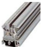
Feed-through terminal block, Connection method: Special and hybrid connection, Number of positions: 1, Cross section: 0.2 mm<sup>2</sup> - 4 mm<sup>2</sup>, AWG: 24 - 12, Width: 5.08 mm, Color: gray, Mounting type: NS 32, NS 35/15, NS 35/7,5
