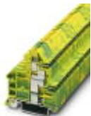
Double-level terminal block, Cross section: 0.2 mm<sup>2</sup> - 4 mm<sup>2</sup>, AWG: 24 - 12, Mounting type: NS 35/7.5, NS 35/15, NS 32, Number of positions: 1, Pitch: 5.08 mm, Width: 5.08, Color: green-yellow
