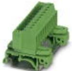
Plug component, Nominal current: 12 A, Rated voltage (III/2): 320 V, Number of positions: 10, Pitch: 5.08 mm, Connection method: Screw connection with tension sleeve, Color: green, Contact surface: Tin, Mounting: DIN rail
