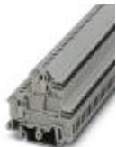
Double-level modular terminal block with COMBICON plug-in zone, nominal current: 12 A, nominal voltage: 250 V, cross section: 0.2 mm<sup>2</sup> - 4 mm<sup>2</sup>, AWG: 24 - 12, mounting type: NS 35/7.5, NS 35/15, NS 32, pitch: 5.08 mm, width: 5.08, color: gray
