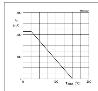
Device mounted on an FR4 printed-circuit board.
