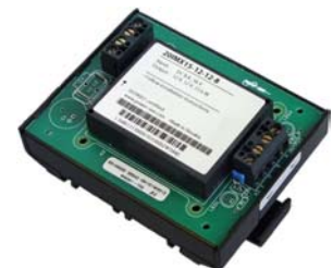
Fig. 24 DIN-rail mounting support HZZ00625.
