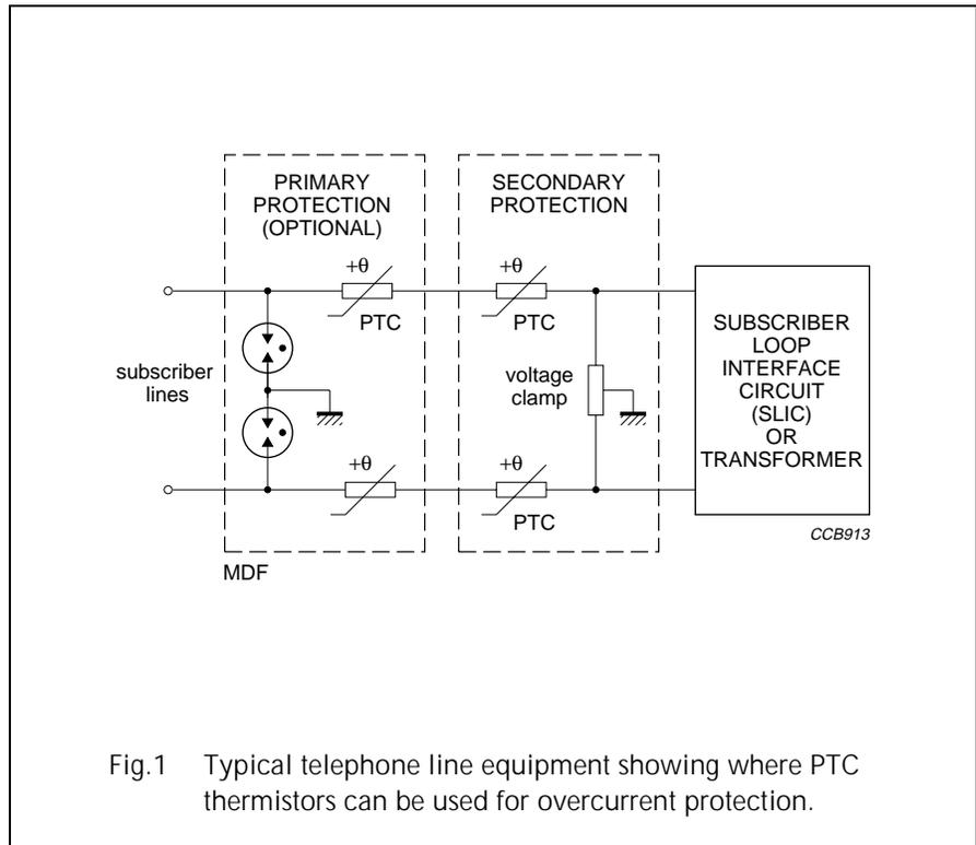
Fig.1 Typical telephone line equipment showing where PTC thermistors can be used for overcurrent protection.
