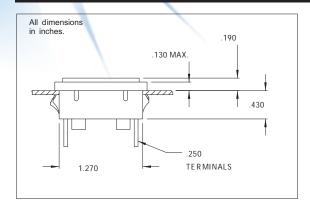
Mounting: Will snap-fit into .032/.100 thick panel, use speednut for other panel thicknesses. Available with speednut SN1963.
