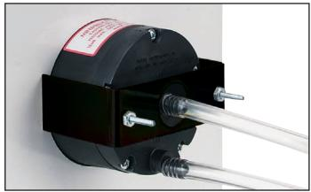
Mounting hardware is supplied with the Minihelic® II gage for panel mounting through a single hole, 2-5/8" (67 mm) in diameter. Panel thickness up to 1/2" (13 mm) can be accommodated with the hardware supplied. If necessary, surface mounting of the gage can be accomplished by means of two 4-40 screws into the tapped mounting bracket stud holes in the rear of the gage. Surface mounting requires clearance holes in the panel for the two pressure taps.
