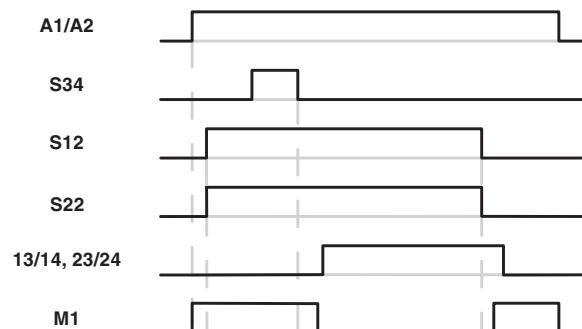
Figure 5 Time diagram for manual, monitored start
