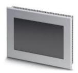
Touch panel with 17.8 cm (7.0") graphics-capable TFT display, 65,535 colors,  $800 \times 480$  pixels,  $1 \times 100$  Ethernet,  $1 \times 100$  MPI,  $2 \times 100$  USB, and integrated runtime of the Visu+ visualization software
