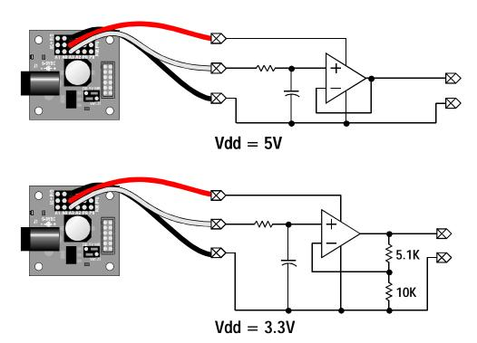
In each case, the op amp should be selected to accommodate rail-to-rail inputs and outputs.
