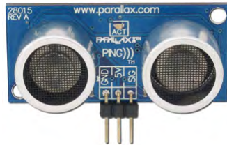
Figure 2-1 The Ping)))™ Ultrasonic Distance Sensor
