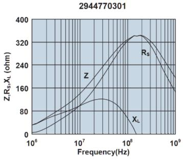
Impedance, reactance, and resistance vs. frequency.
