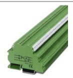
Input solid-state relay, with DC voltage output push-pull, transmission frequency: 100 kHz, with light indicator and protective circuit in input and output circuits, input: 5 V DC, output: 14 - 30 V DC/50 mA
