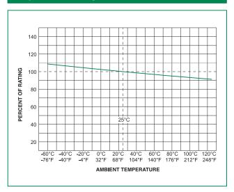
1. Derating depicted in this curve is in addition to the standard derating of 25% for continuous operation.
