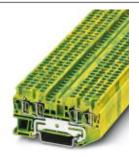
Ground modular terminal block, connection method: Spring-cage connection, number of connections: 4, cross section:0.08 mm² - 4 mm², AWG: 28 - 12, width: 5.2 mm, color: green-yellow, mounting type: NS 35/7,5, NS 35/15
