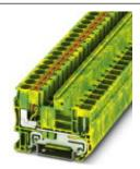
Ground modular terminal block, connection method: Push-in / plug connection, number of connections: 2, cross section: 0.5 mm² - 10 mm², AWG: 20 - 8, width: 8.2 mm, color: green-yellow, mounting type: NS 35/7,5, NS 35/15
