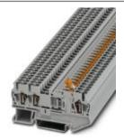
Knife disconnect terminal block, Connection type: Spring-cage connection, Cross section: 0.08 mm² - 4 mm², AWG: 28 - 12, Nominal current: 20 A, Nominal voltage: 400 V, Length: 72 mm, Width: 5.2 mm, Color: blue, Assembly: NS 35/7,5, NS 35/15
