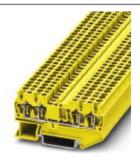
Feed-through terminal block, nom. voltage: 800 V, nominal current: 24 A, connection method: Spring-cage connection, number of connections: 4, cross section:0.08 mm² - 4 mm², AWG: 28 - 12, width: 5.2 mm, color: yellow, mounting type: NS 35/7,5, NS 35/15
